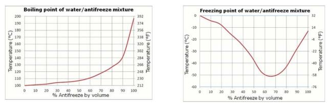
The coolant/antifreeze used at first fill is chosen by the vehicle manufacturer as the most suitable. Subsequent service top ups or renewals should use a product meeting the original specification so the vehicle warranty is not affected.
