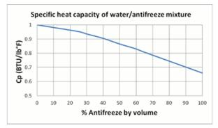
the mixture. While water provides the best heat transfer, glycol is also used in coolants to provide freeze protection.
